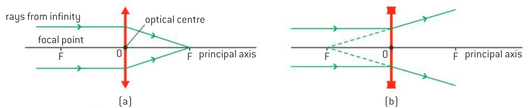
▲ Figure C.1.3. The terms for a (a) converging lens and (b) a diverging lens
